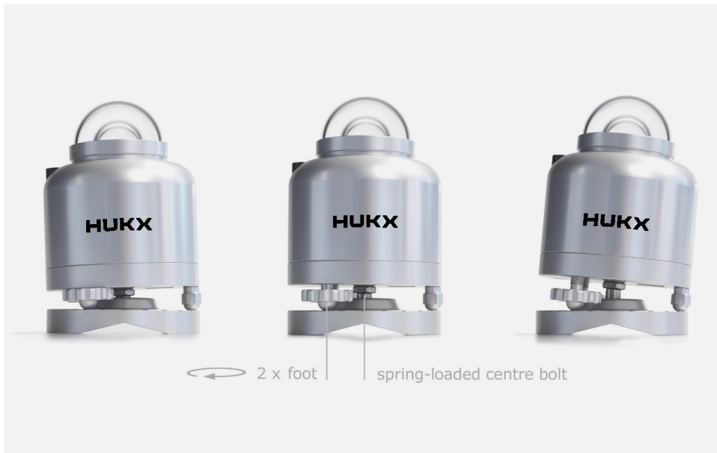
Figure 5.3.6.1.5 Pyranometer locked on its optional leveling mount: by fastening (on the left) or loosening (on the right) the two adjustable feet, the pyranometer can be levelled, using the bubble level as a reference. The static foot remains fixed. In all cases, ensure the legs of the pyranometer fit into one of the small ledges of the leveling mount. Locking is in place, when the nut is turned all the way against the bottom plate of the pyranometer.
