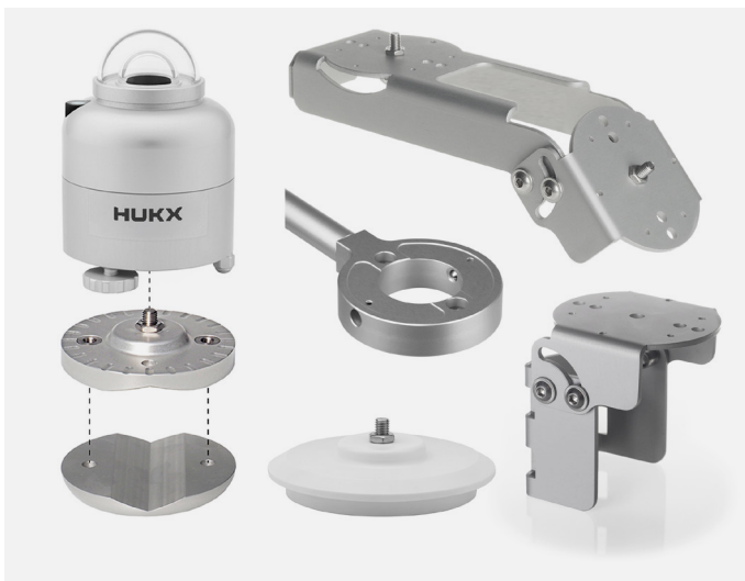
Figure 0.8 Examples of optional accessories for the most common ways to mount and level pyranometers, and also to electrically insulate them from their metal mounting platform.
