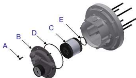
Fig 9.6 - Separator Element Location
