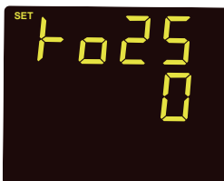
Fig 3-34 RO2 Alarm Inequality Setting
