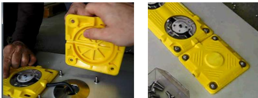
Figure 26 - Installed Cable Bushing
