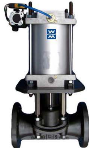
Above: 100mm DIN 3202F1 cast iron body, ebonite lined pneumatically actuated diaphragm valve coupled with a 200mm double acting pneumatic air cylinder and air booster.
