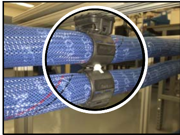
Figure 4 Two hoses connected to a single RediFlex II frame bracket.
