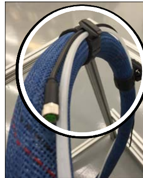
Figure 5 Solenoid tubing and a signal cable routed through the RediFlex II hose hanger.
