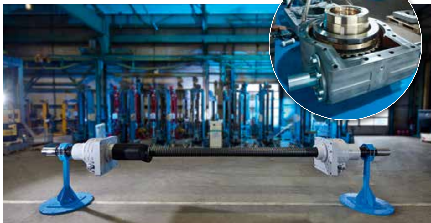
Assembly area PFAFF-silberblau: Special design screw jack SHE 200.1 with 8 m long screw and protection boot. Design for a static load of 400 tons.
