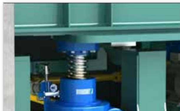
Pfaff-silberblau – 500-ton lifting unit for the adjustment of zinc furnaces
