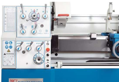
The user-friendly control panel at the headstock facilitates rapid user familiarization and intuitive operation
