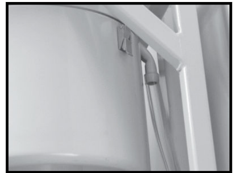
Step 6. Fit oil return hose and position tube to drain oil back to machine enclosure, sump or collection vessel.
