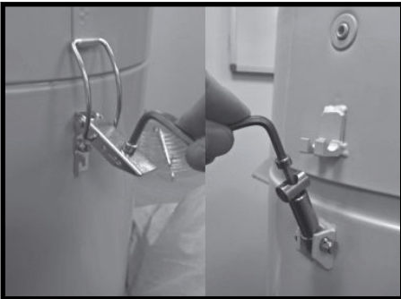
Step 1. Undo safety latch and clips.
