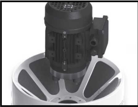
Step 13. Re-fit motor to top of case.
