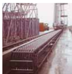
BS 3500 steel chains with supporting frame applied to De lcing's equipment at München airport (Germany).
