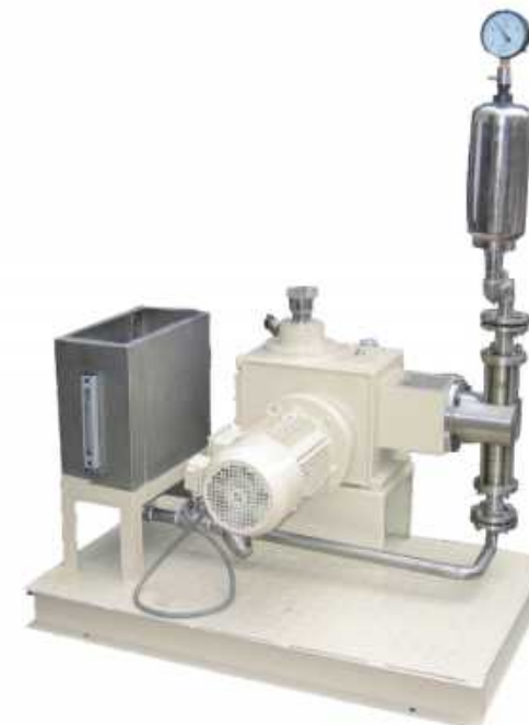
■ Pump Skid With Damper
