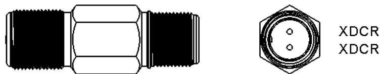
Figure 9 – MS Connector Pickoff Wiring: Pickoff codes -1 (RF) and -2 (MAG)
