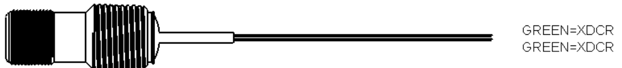
Figure 11 – Explosion Proof, Flying Leads Pickoff Wiring Pickoff codes -X3 (Explosion Proof MAG) and -X5 (Explosion Proof RF)
