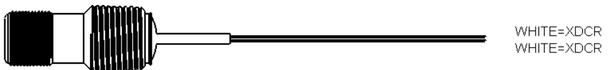
Figure 10 – Flying Leads Pickoff Wiring: Pickoff codes -3 (MAG) and -5 (RF)
