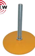
Part. R0408 - Pag. R43 Ø 160 • Painted steel • Max. load 50000 N.
