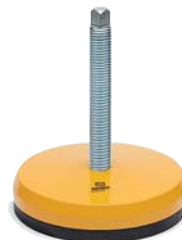
Part. R0406 - Pag. R55 Ø 123 • Painted steel • Max. load 50000 N.
