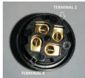
Pin detail for Field Wireable Connector
