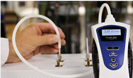
Figure 4: Probe connected to a GC gas outlet.
