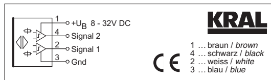
Fig. 21 Terminal diagram BEG 53A/BEG 54A
