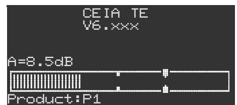
After the alarm, the maximum signal is visualized for a few seconds together with its amplitude
