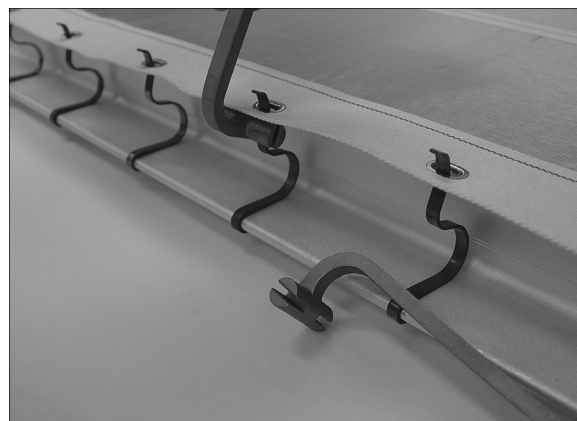
3.6. Discharge End of Screen Frame with Edging Pulled Down on Clips
