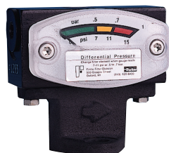
DPG-15HP Differential Pressure Gauge Temp: 200°F (93°C) Pressure: 800 PSIG (55 bar) (Fits on pre-drilled M-Series housings only)
