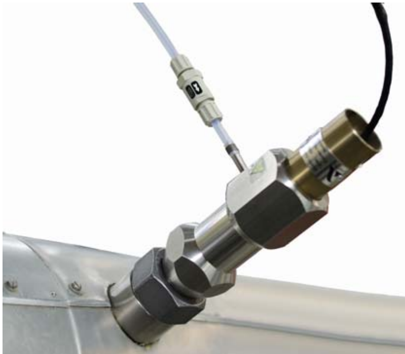
Fig. 9-3 Testing device plugged into flue gas channel
