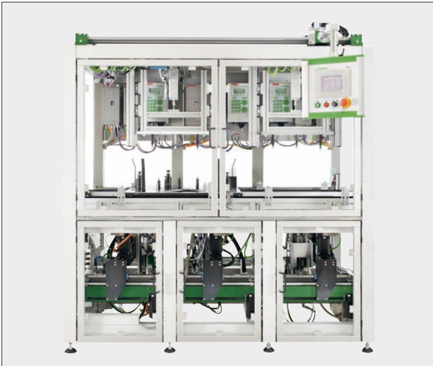
Conveyor-integrated screwdriving station for the inverted assembly of electric motors.
