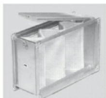
IFL-G4 Filtration box with IFR-G4 filters incorporated Casing manufactured from galvanised sheet steel and provided with G4 filter type. Supplied with standard rectangular flanges. Access door to ease filter replacement. Can be fitted in any position. Working temperature up to 80°C. Maximum recommended differential pressure.
