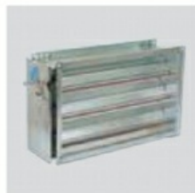
IJK Damper Supplied with standard rectangular flanges. Manufactured from galvanised sheet steel. Fitted as standard with removable handle. Shaft diameter: 10 mm. As accessory: electrical damper actuator LM230A.
