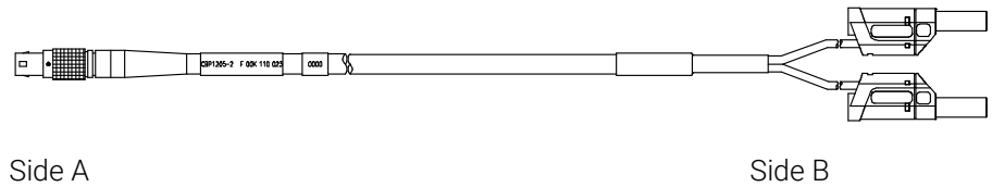
Fig. 9-2 Cable CBP1205 (power supply cable with safety banana plugs)
